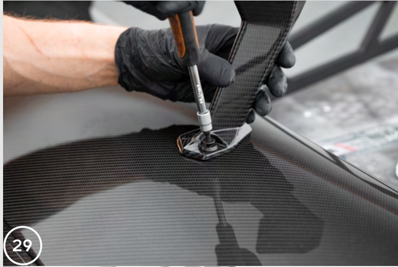
31. Place the spoiler and brackets on the tailgate. Screw the spoiler brackets to the tailgate using the holes drilled on the edge of the tailgate. If there are differences in the positions of the mounting holes and the drilled holes, we recommend enlarging the drilled holes so that the spoiler brackets rest completely on the tailgate.
