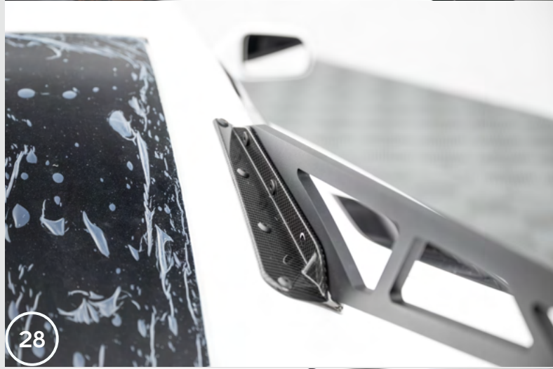
31. Place the spoiler and brackets on the tailgate. Screw the spoiler brackets to the tailgate using the holes drilled on the edge of the tailgate. If there are differences in the positions of the mounting holes and the drilled holes, we recommend enlarging the drilled holes so that the spoiler brackets rest completely on the tailgate.
