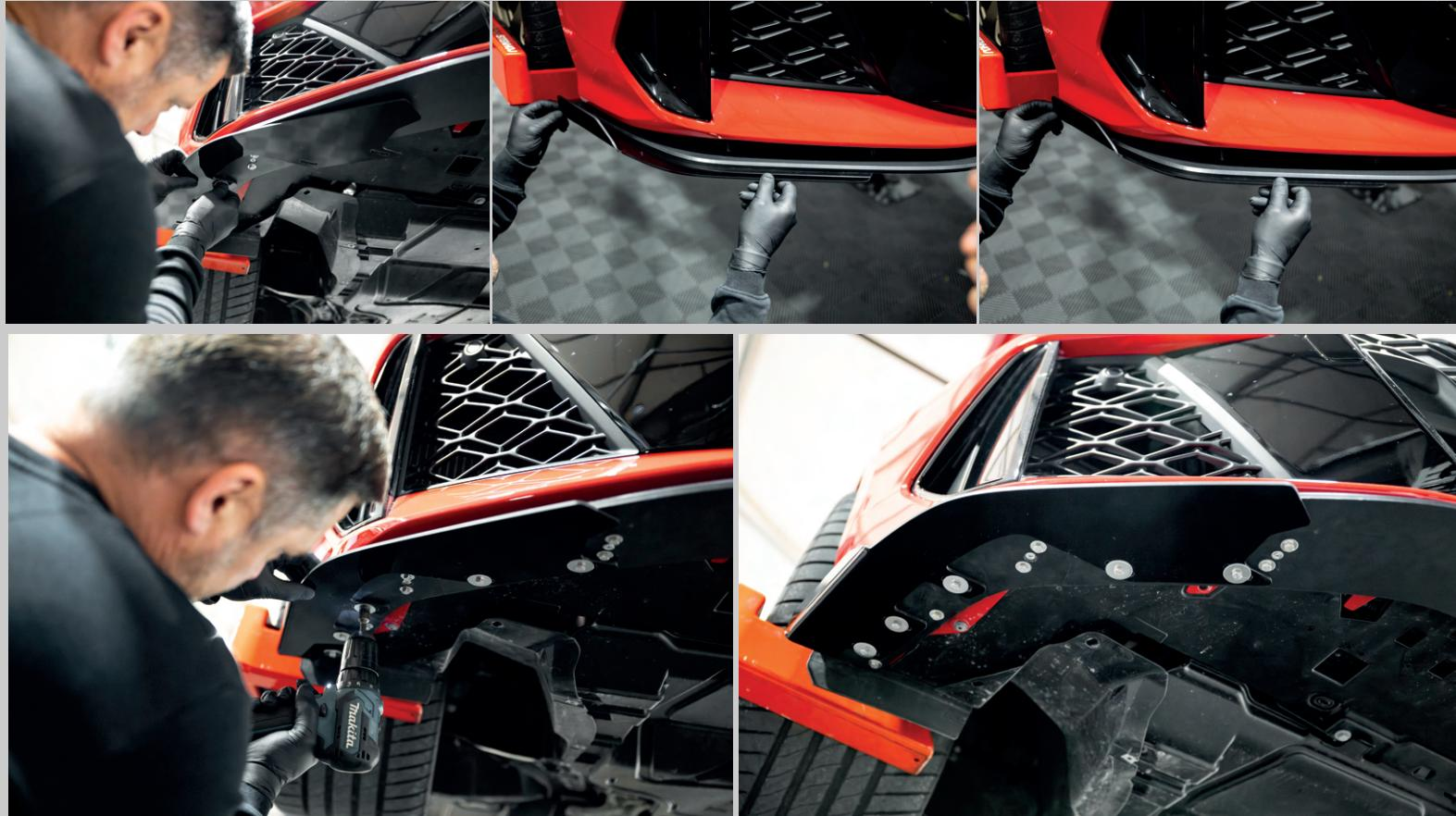
Place the flaps on the splitter so that the holes in the flaps line up with the threads in the splitter. Lightly screw the flaps to the splitter. Determine how much your flaps should stick out behind the splitter. Then tighten the bolts fastening the flaps tightly. Ready.
