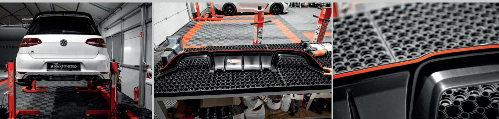
Before installation, pay attention to what type of rear valance you will be installing. A glued-in rear valance is characterized by the fact that double-sided tape is placed on the inside of the rim, and the valance does not have any mounting tabs. Before installation, wash and dry the car. We recommend using lifts. At least 2 people are needed.
