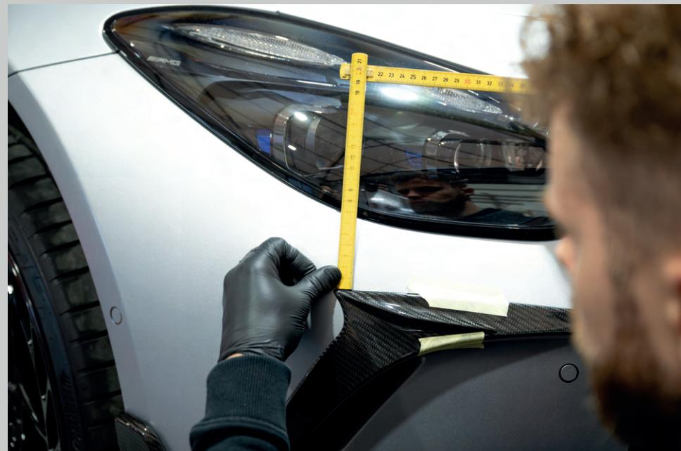
Align the canards on both sides of the bumper. The distance of the canards to the grill and to the lamp line should be the same on both sides of the bumper. We recommend measuring the distance so that the applied tape measure indicates the distance straight ahead from the canards.
