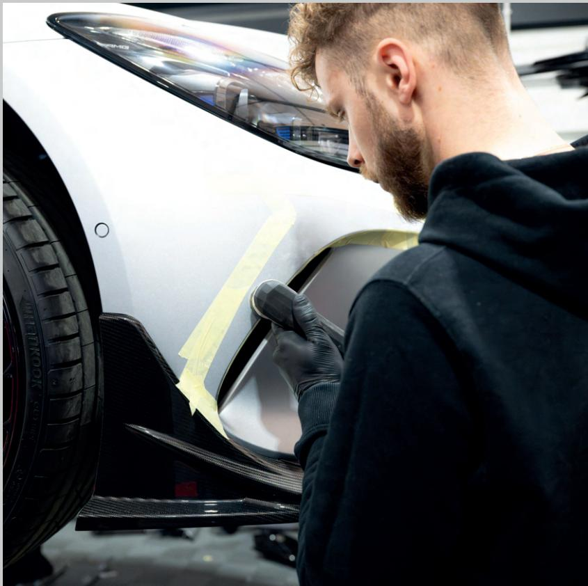
After positioning and aligning the canards, use masking tape to mark the outline of the canards on the bumper. This should be done carefully so that you can accurately determine their final position later on.
