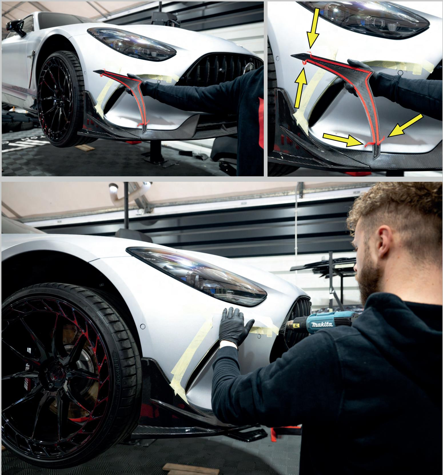
Remove small pieces of protective film from the double-sided tape placed on the canards and bend them outwards. Using a heater, gently warm up the surface where the canards are mounted, being careful not to damage the surface.
