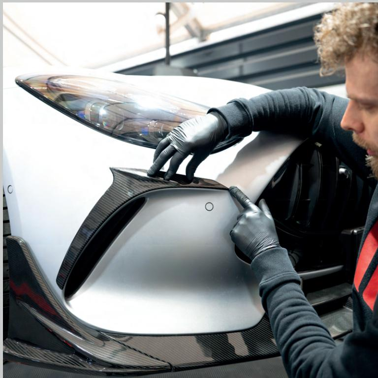
Place the canard on the bumper at the embossment under the lamp. Place the canard so that its shape matches the embossment line on the bumper. The canard should be placed so that the embossment line is visible from the bottom of the canard.
