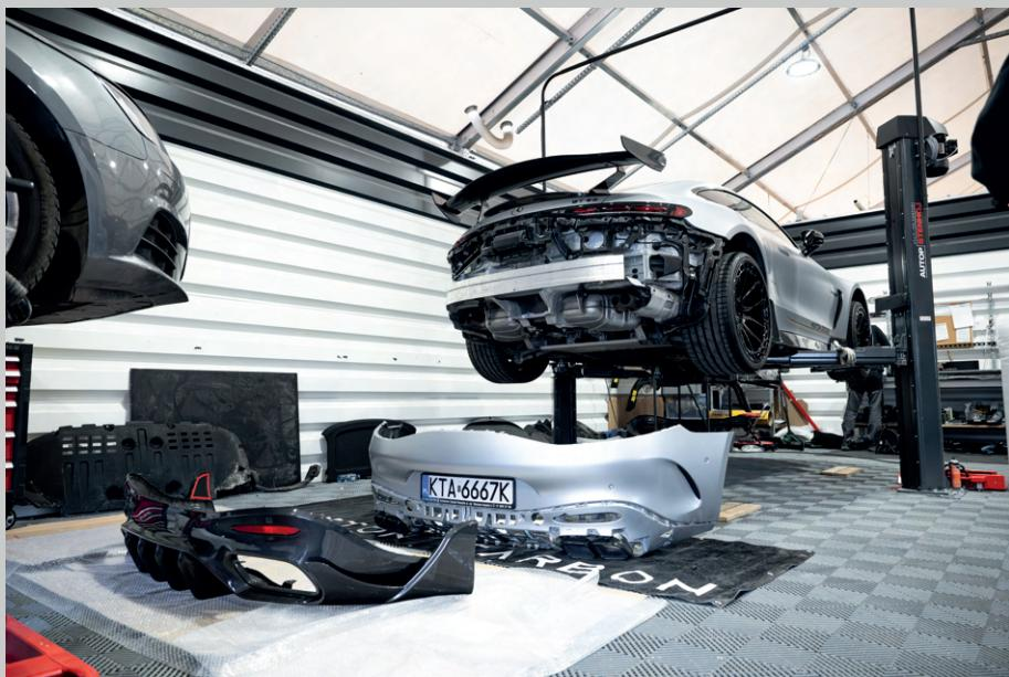
Before installation, the car should be clean and dry. We recommend using jacks. Before installation, remove the original diffuser, disconnect the electrical connectors and remove the bumper.
