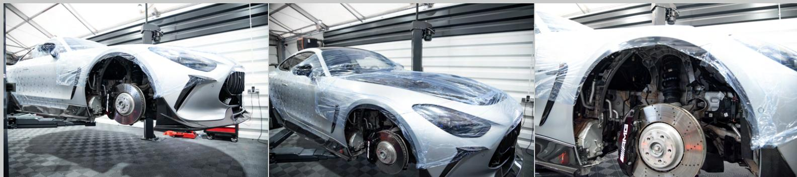
Before assembly, remove the front wheels of the car and the wheel arch covers. Secure the front of the car. We recommend working with two people. The car should be clean and dry.
