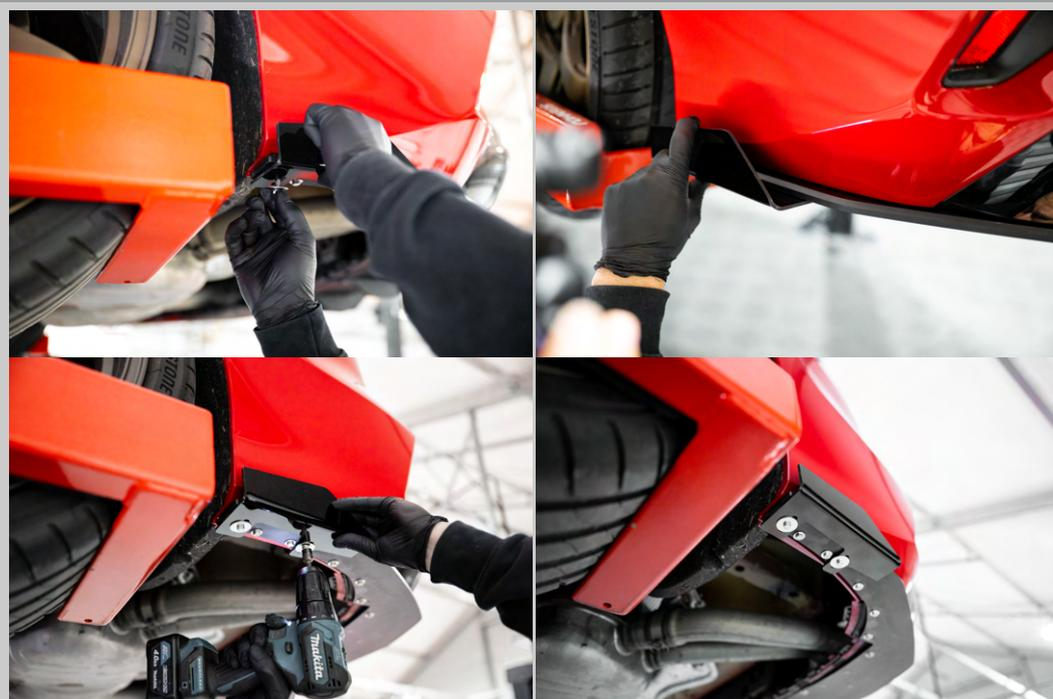
Place the rear side flaps against the rear diffuser where the thread is visible. Then screw the rear side flaps lightly using the screws from the assembly kit. Determine how much the rear side flaps should protrude from the diffuser. Then screw the rear side flaps tightly. Done.
